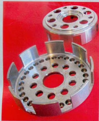
A selection of uprated Vespa clutch components: billet additional-spring baskets for old-style PX and P2/T5 clutches.
