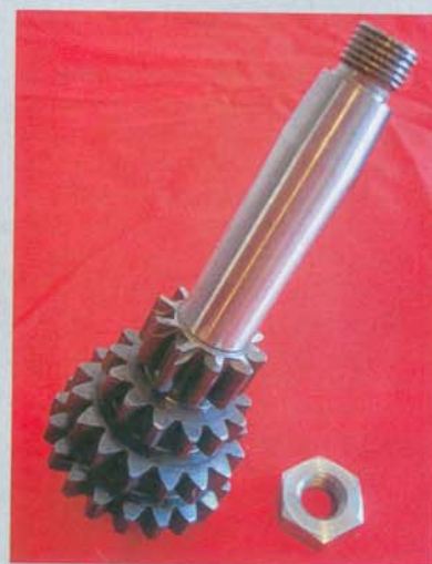
The new smallframe Nurburg gear cluster has a special 11 mm x 1 mm thread. The special clutch nut can now be tightened to 9kgm instead of the standard figure of 4.5kgm.
