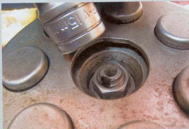
DRT's genius Vespa largeframe clutch nut eliminates the need for those hideous castle nuts. And all those trips to casualty when the peg tools slip.
