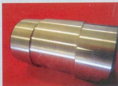
DRT's eccentric crankpins can be used to increase crankshaft stroke.
