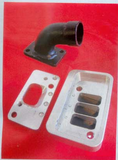
Prototype reed valve conversion for large frame Vespa engines.
