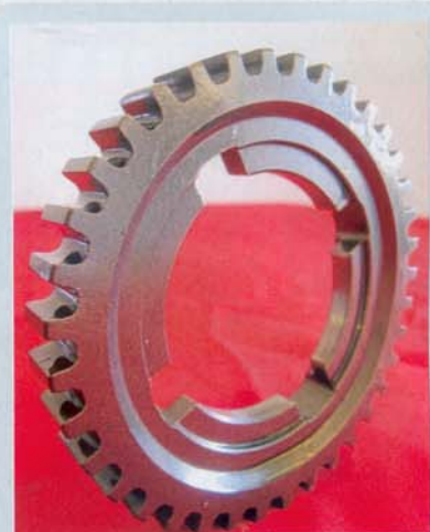
One of DRT's many different interchangeable loose gears. Special tooth profiles allow cogs with different numbers of teeth to mesh with the same gear cluster.
