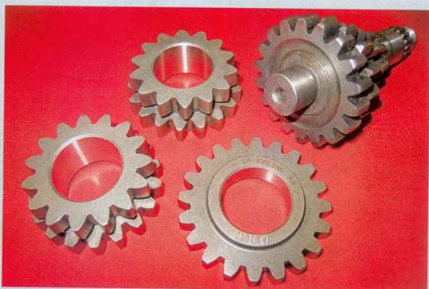
A selection of DRT cogs that can be pressed onto a specially-modified Lambretta gear cluster in order to create a close ratio gearbox.
