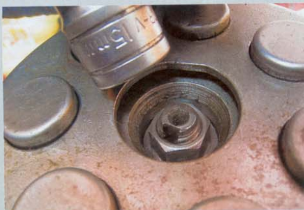
DRT's genius Vespa largeframe clutch nut eliminates the need for those hideous castle nuts. And all those trips to casualty when the peg tools slip.
