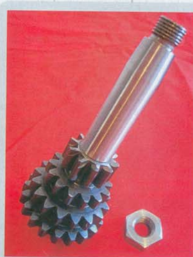
The new smallframe Nurburg gear cluster has a special 11 mm x 1 mm thread. The special clutch nut can now be tightened to 9kgm instead of the standard figure of 4.5kgm.
